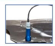
Measurement of hydrogen flux from a metallic surface for corrosion monitoring.
