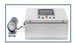
Diffusible hydrogen content measurements according to the draft ASTM WK47776.
