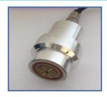
Measurement of diffusible hydrogen content on the inservice products. Avoiding the component cutting and the coating removal.
