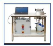
Hydrogen Permeation Tests according to EN ISO 17081:2014, ASTM G148-97 (2018) & EN10209:2014(2018).
